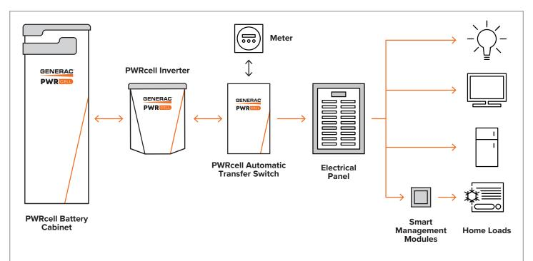
The ATS and SMMs allow installers to prioritize loads in the home, preventing system overload. PWRcell can manage power distribution to essential and non-essential loads in the same panel, shedding non-essential loads when necessary and re-powering them when able.
